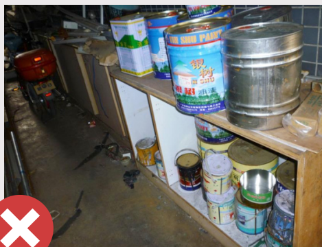
Poor storage of flammable liquids.
